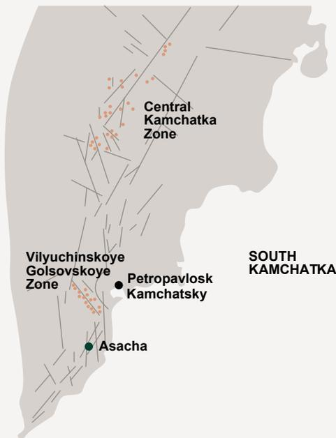
An epithermal gold/silver deposit located on a tertiary volcanic arc typical of ore systems found along the Pacific Rim. The main ore zone at Asacha consists of five steeply dipping veins with two principal veins averaging over two metres in width. Veins are characterised by low sulphidation quartz-adularia occurring predominately in dacite domes.
